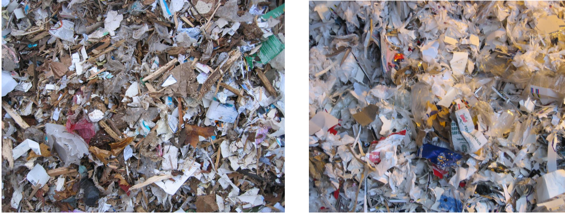
Figure 7. Waste wood (left, containing occasionally also paper and plastics) and SRF fractions at the Kauttua plant.
