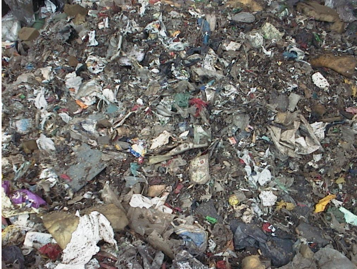
Figure 5. The shredded fuel as fed into the boiler at the Norrköping waste-to-energy plant.
